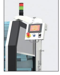
CONTROL PANEL ON 180-DEGREE ROTATING ARM
